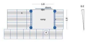
s = Existing concrete slabs d = existing drain cover dpc = damp proof course r = railings
